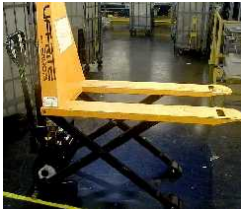
Lifter-transporter — a combination pallet jack and powered scissors lift
